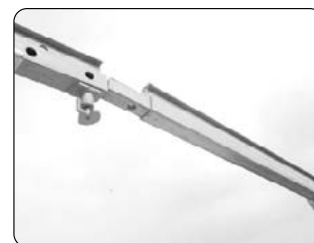
Kupplung der Schienensegmente Coupling for the rail segments
